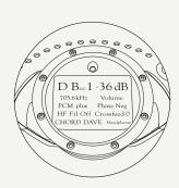
\*DAVE will only display Dual BNC when BLU MK llis transmitting a 768kHz or 705.6kHz signal. Therefore BLU MK II must be set to maximum upsampling which is denoted by the white button colour.
