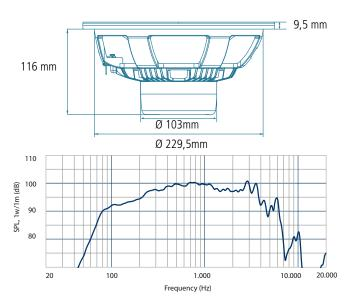
Frequency response curve of the loudspeaker make in a hemispherical, free field and mounted in a reflex box with an internal volume of 50 litres and tuned at 60Hz, applying a sinusoidal signal of 2.83 V @8 at 1m.
