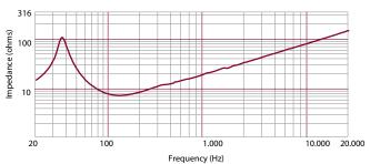
Impedence magnitude curve measured in free air
