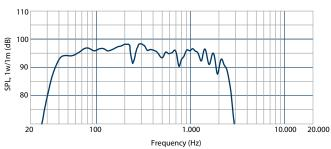
Frequency response curve of the loudspeaker make in a hemispherical, free field and mounted in a reflex box with an internal volume of 55 litres and tuned at 60Hz, applying a sinusoidal signal of  $2.83 \lor @8$  at 1m.
