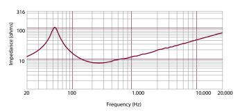
Impedence magnitude curve measured in free air
