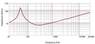
Impedence magnitude curve measured in free air
