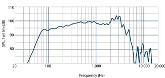
Frequency response curve of the loudspeaker make in a hemispherical, free field and mounted in a reflex box with an internal volume of 55 litres and tuned at 60Hz, applying a sinusoidal signal of 2.83 V @8 at 1m.
