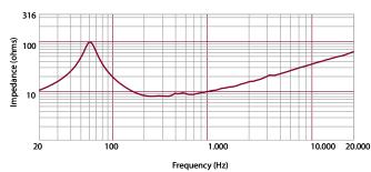
Impedence magnitude curve measured in free air
