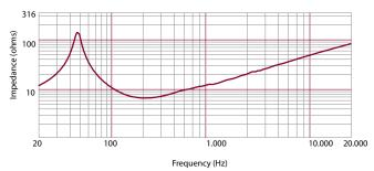
Impedence magnitude curve measured in free air
