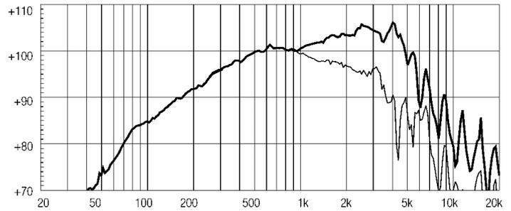
**FREQUENCY RESPONSE CURVE OF 10NDA610 (AIC ON) MADE ON 30 LIT. CLOSED ENCLOSURE IN FREE FIELD (4PI) ENVIRONMENT. ENCLOSURE CLOSES THE REAR OF THE DRIVER. THE THIN LINE REPRESENTS 45 DEG. OFF AXIS FREQUENCY RESPONSE.**
